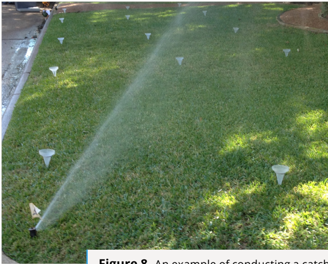
Figure 8. An example of conducting a catch can test to measure the precipitation rate.
